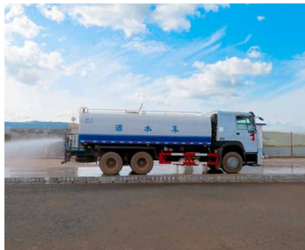
Road water-sprinkling dustfall of the Souapiti project in Guinea
